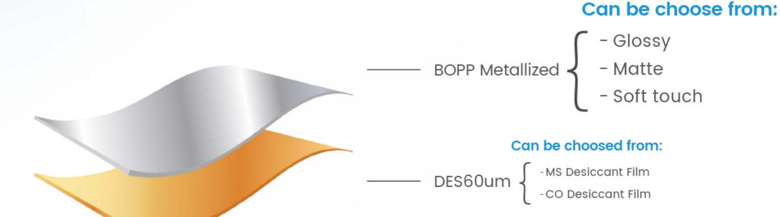
WiseFlex+ Recyclable Desiccant Film is a composite functional film primarily made from PP. To enhance light blocking, a small amount of metallization is applied, which does not affect recyclability. The desiccant layer provides self-moisture absorption, effectively controlling humidity and protecting the packaged products from moisture damage, thereby extending shelf life.
