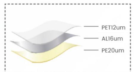
WiseForm+ is used in conjunction with WiseLid seal foil or child-resistant seal foil for a more secure seal. WiseForm+ and WiseLid are combined products, and currently, WiseForm+ standard products are not sold separately.
